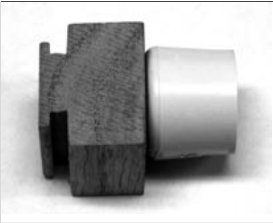
Homemade hot shoe adapter attached to CPVC cap
